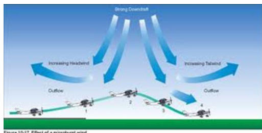
Figure 10-17. Effect of a microburst wind.
